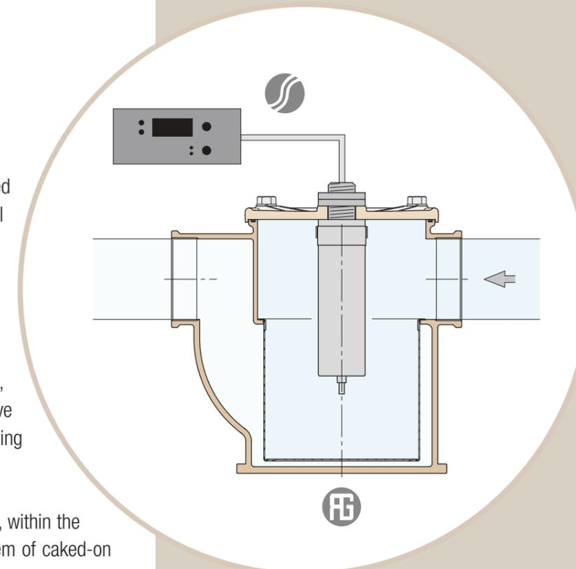
fouling, eliminating the risk of organic marine deposits: the modular control unit makes it possible to work at a lower amperage and can be interfaced with other electronic systems on-board.
